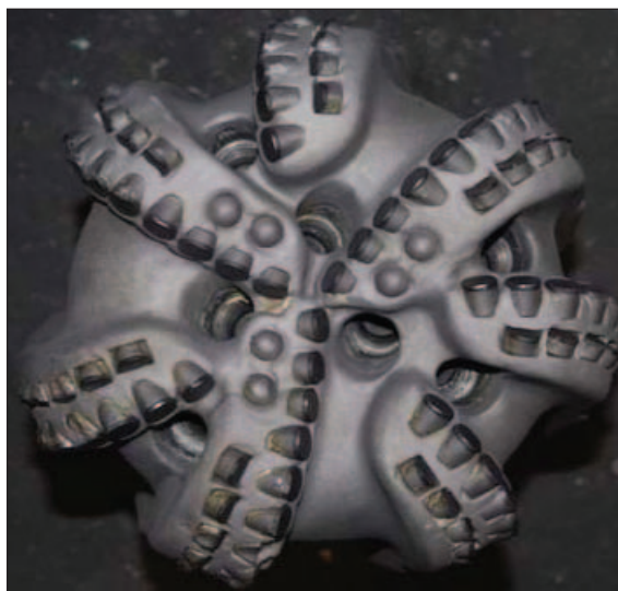
The post-run analysis of the 9 \frac{7}{8} -in. DE713PUX Diamond Edge bit confirmed the durability of the cutting structure in the Haynesville shale. (Image courtesy of Varel)
