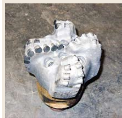
Fig. 5. The proprietary four-blade bit that drilled the entire 6,570 ft of a 7 7/8-in. interval in one of the operator's Piceance Basin wells was graded as "1 1 CT C X I NO TD."
