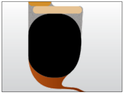
Heat shield ring with a conical seal gland helps prevent thermal degradation of the seal
